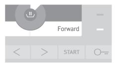
▶ Press button Open the door (is not lit!). The programme will be interrupted and the door unlocked.
