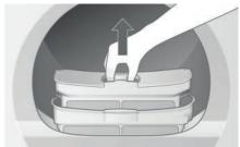
Pull out the inner, fine filter A and swing it open.
