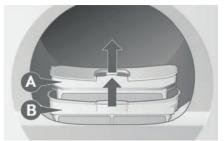
Pull both filters out of the filter support.
