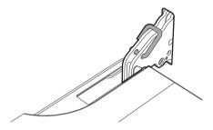
2. Grasp the door on both sides with both hands, lift it forming an angle of around 30° and remove it.
