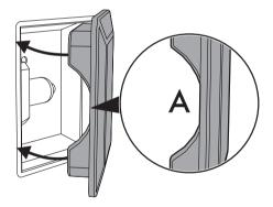
Press the cover completely down so that it attaches perfectly to the bulb support.
