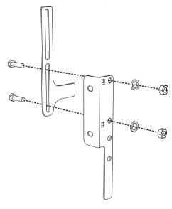
4. Align the base of the hook on the fastening bracket with the base of the slot on the wall fastening plate.
