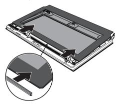
5. Remove the intermediate glass pane by lifting it upwards.
